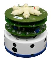
Fig. 3. The Khepera IV robot with custom relative position, odor and wind measurement extension boards.
